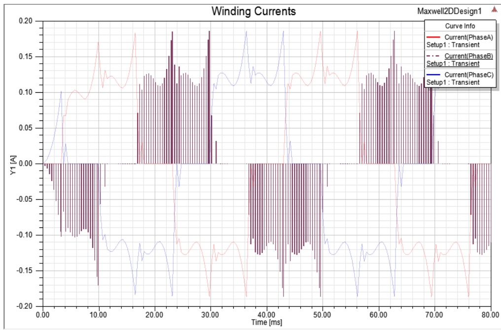
Figure 11.0: Simulated BLDC performance under Trapezoidal commutation with respect to reactance in phase B
